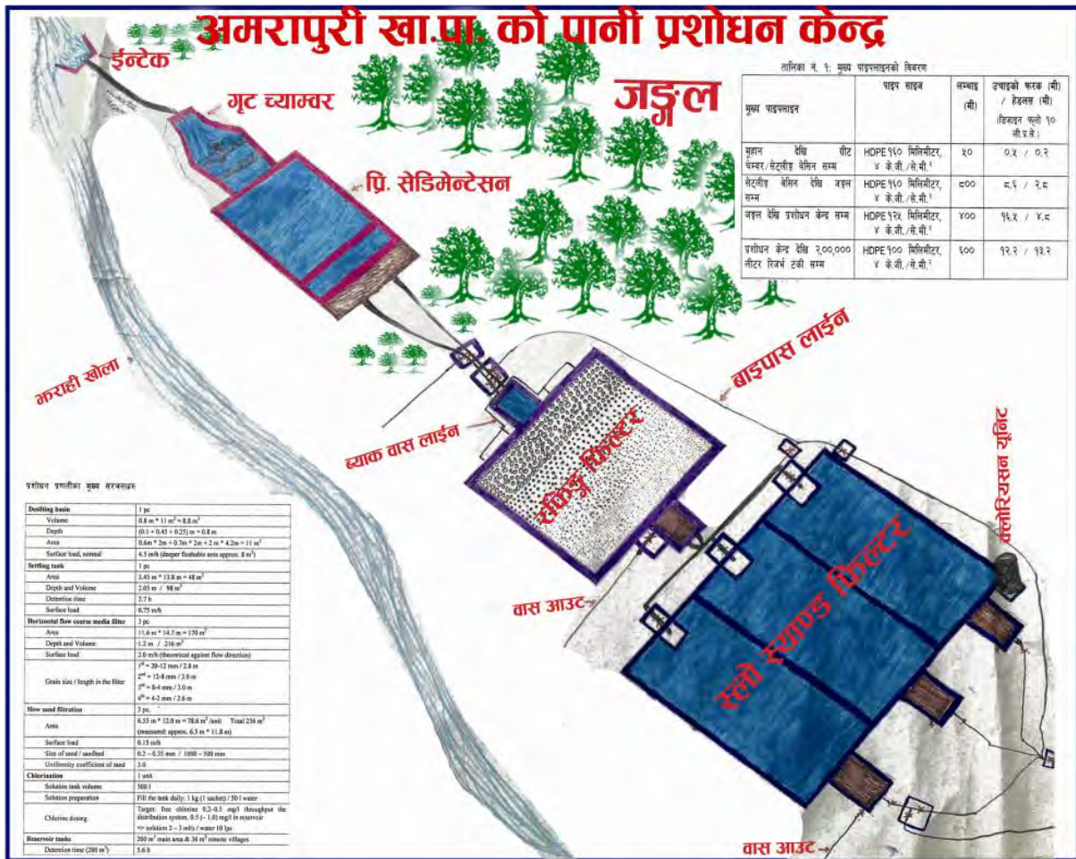
Figure 21 Amarapuri water-supply system schematic
