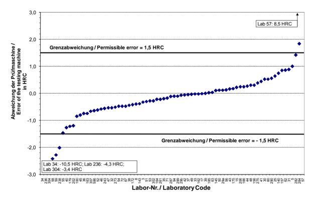
Figure H.1: Test A, Example 45 HRC-Level: Error of the testing machine
