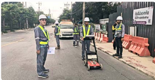
Proactive Risk Mitigation: MWA advances trunk main leak detection and soil density survey across Samsen Road; No anomalies detected
